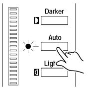
Depress the appropriate Exposure Adjustment Button, either LIGHTER or DARKER, to set the desired image density, or exposure, level.
